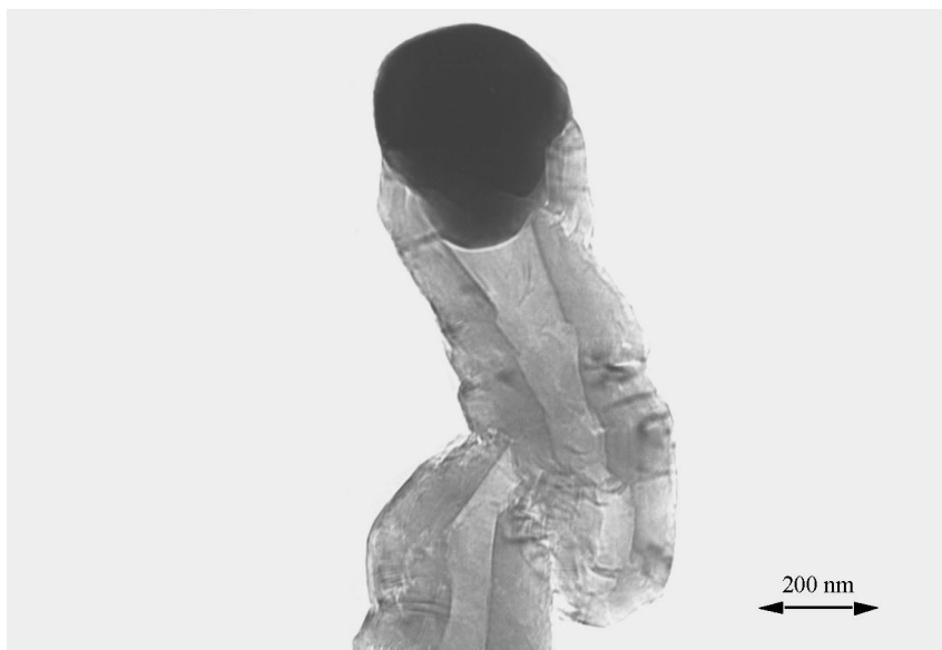
Fig. 14. Transmission electron micrograph showing the appearance of a carbon filament and the associated catalyst particle produced after reaction at 865°C with an \text{C}_2\text{H}_6/\text{H}_2\text{O} (4:1) mixture containing 150 ppm \text{H}_2\text{S} .
